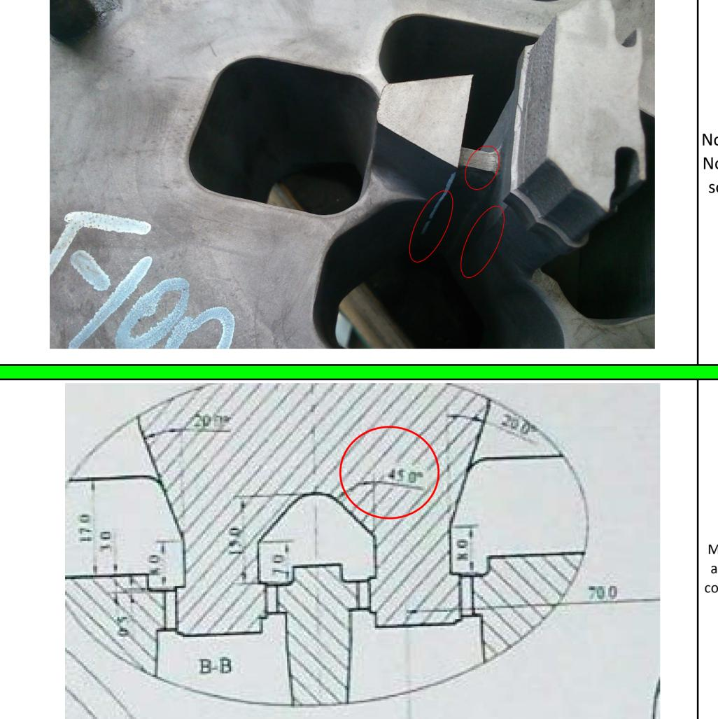
No sharp edges!! No good support so the Mandrel can move!
